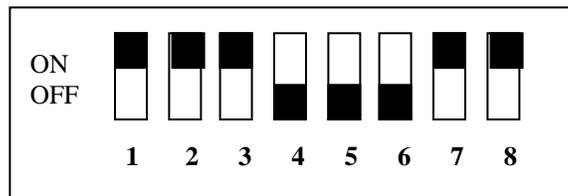
DB Sensor settings (smaller unit) dip switches 1 thru 6 are set at the factory and only need to be changed if your neighbor has a DB200 or DB100. The 8 dip switches should be set as follows:
